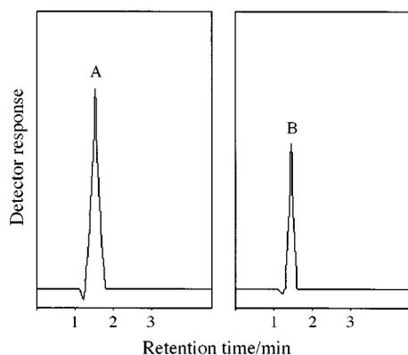
Fig. 1 Chromatograms showing, A, an oil sample and B, an MDA standard.
